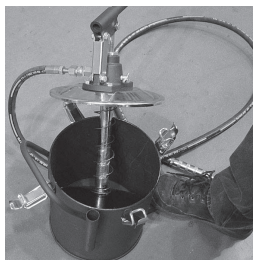
Grease Pump with Drum Cover removed
